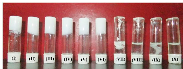
Figure 2. CuCl 2 –thiourea complex as metallogel with variation in CuCl 2 molar equivalent from 1.0–0.1 w.r.t. molar equivalent of thiourea (From set I to set X).
